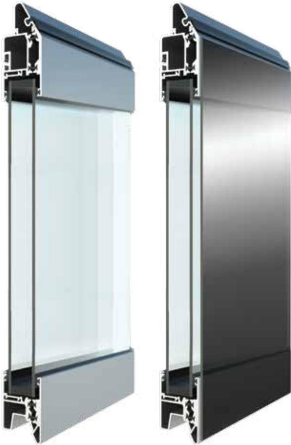
Aluminium profiles with thermal break significantly upgrade the insulation value of a panoramic sectional door panels. FV Thermo doors are produced up to 7 meters wide, 6 meters high, with standard double panes of acrylic glazing or double Anti-Scratch glazing. Concerning possible measurements of doors, glazed with double Safety Glass — consult the factory.
